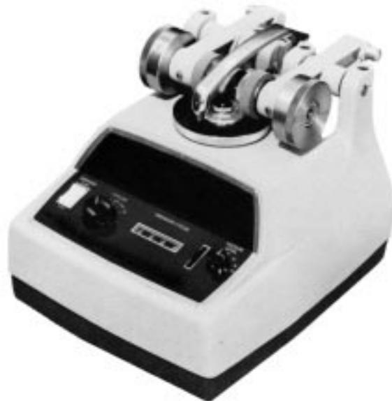
**FIG. 1 Rotary Platform Double Head Abrader**
